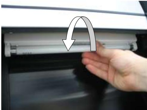
Fluorescent tube to be used: OSRAM L 8W/840 25X1 or comparable
