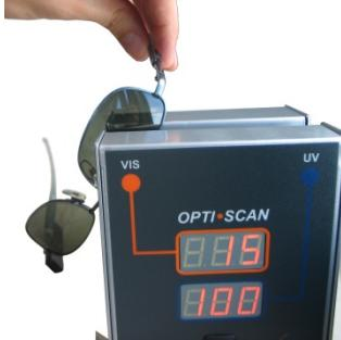
Transmission des UV-LichtesTransmission of visible light (VIS)Transmission of UV lightTransmission de la lumière visibleTransmisión de la luz visible (VIS)Transmission de la lumière uvTransmisión de la luz UV
